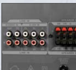
The I/O panel found on the rear of the subwoofer
