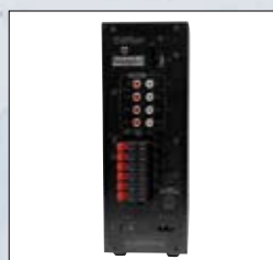
All inputs, including USB and SD card slot are on the reverse side
